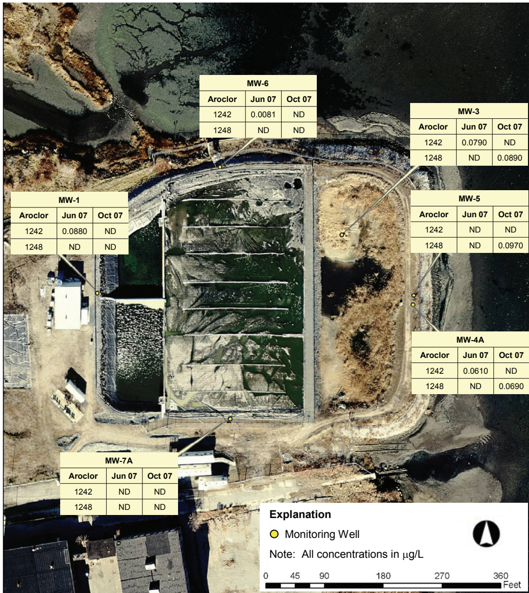
Figure 1: Sawyer Street CDF Monitoring Well Locations and PCB Aroclor 1242 and 1248 Concentrations in Groundwater
