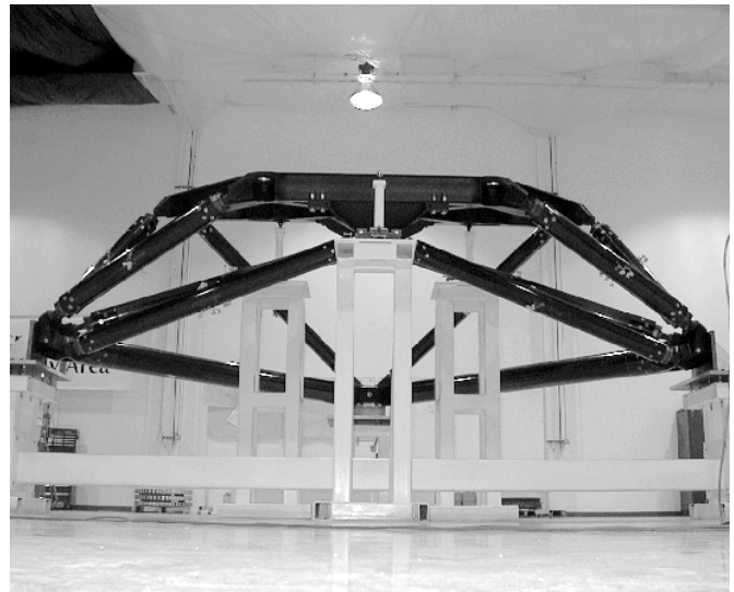
The Forward Structural Adapter is designed to mate the Deorbit Propulsion System to the body of the X-38, locking the Crew Return Vehicle’s propulsion system into place.
