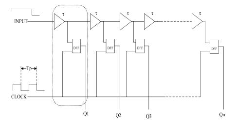
Figure 2. Tapped delay line made of slices.
