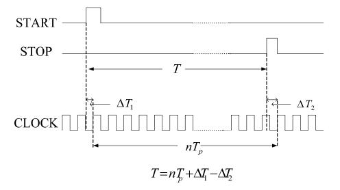
Figure 1. Interpolating Principle
