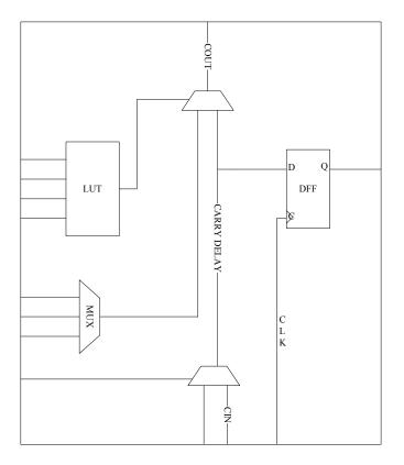
Figure 3. Simplified slice configuration as delay unit.
