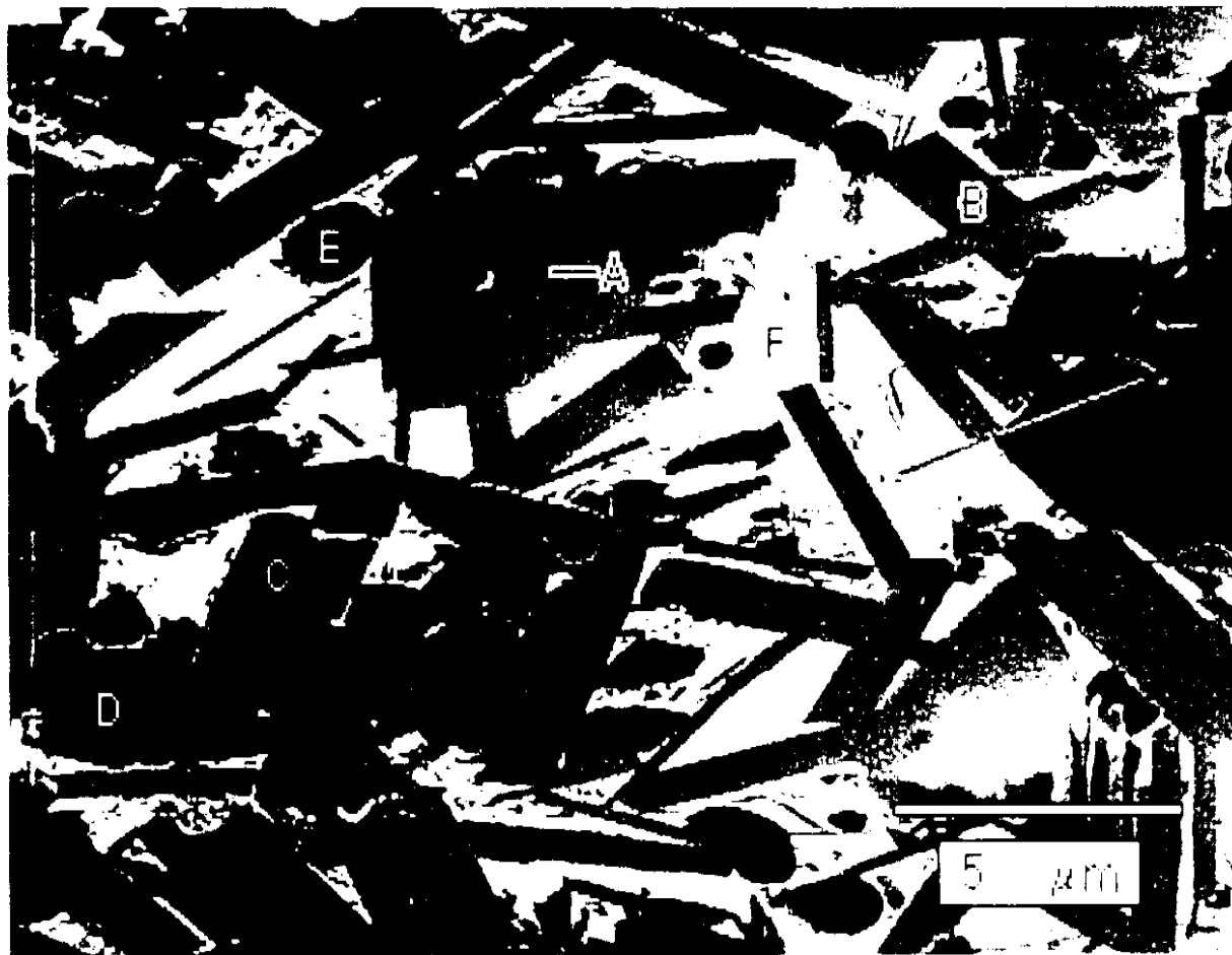
Fig. 10. Backscattered electron micrograph, showing microstructure of composition 2 quenched from 980 °C. A = residual 1223; B = 1212; C = (\text{Sr,Ca})_2\text{CuO}_3 ; D = (\text{Ca,Sr})\text{CuO}_2 ; E = (\text{Ca,Sr})\text{O} ; F = melt.
