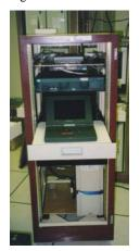
Figure 3. Mobile Router Rack
