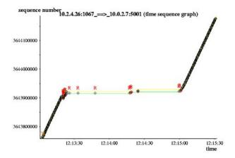
Figure 7. TCP transfer with Hold down Timer = 30 sec
