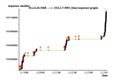
Figure 6. TCP transfer with Hold down Timer = 0
