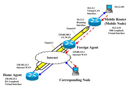
Figure 1. Mobile Router Tunneling
