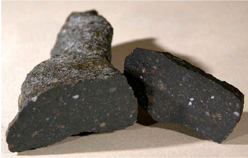
Figure 1: Dhofar 1180 illustrating dark glassy matrix and light colored feldspathic clasts. Image from M. Farmer. Width of sample is 8 cm.
