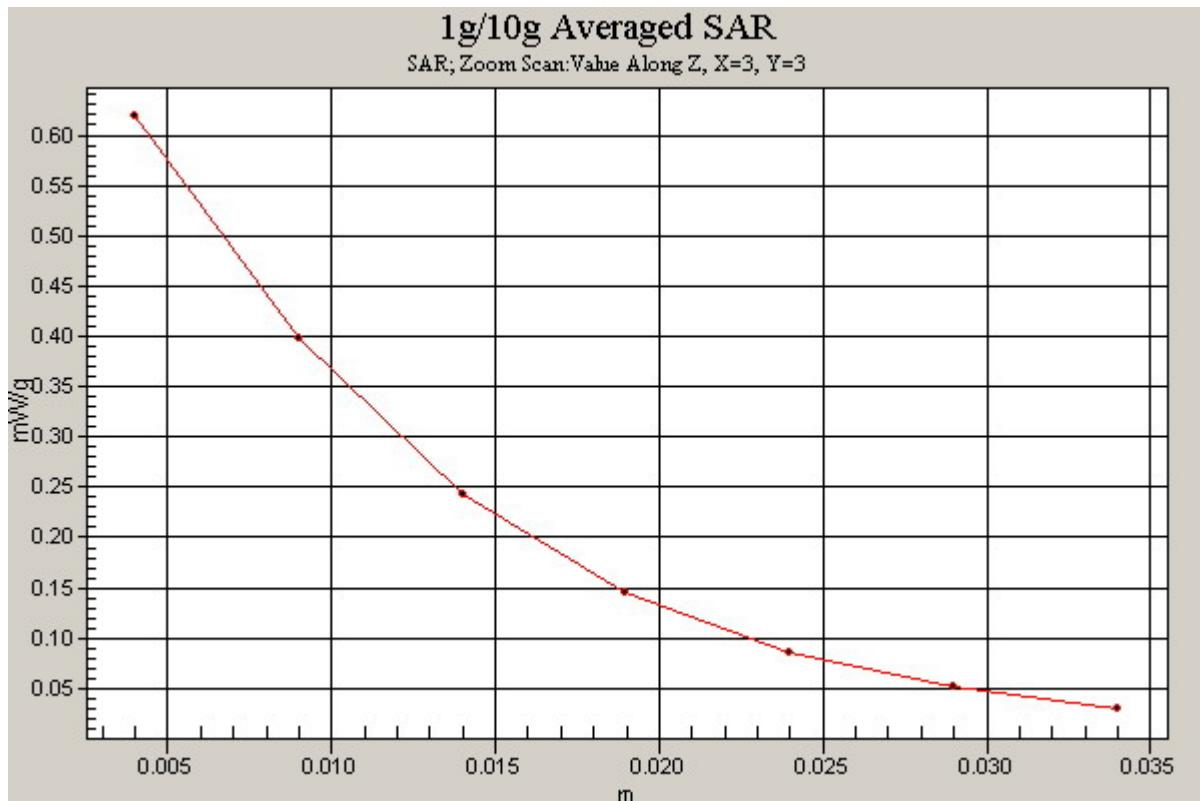
**Figure.18 Z-Scan at power reference point (Left Hand Tilt 15° CDMA PCS Channel 25)**
