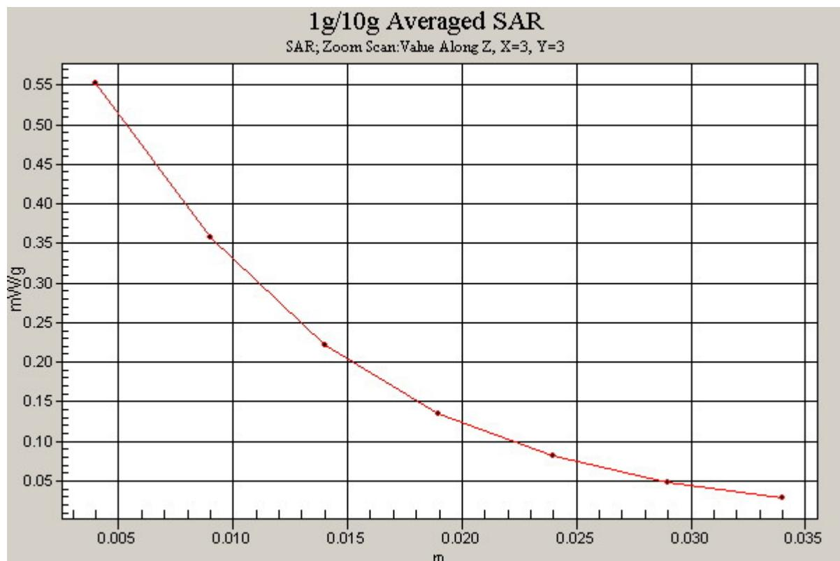
**Figure. 26 Z-Scan at power reference point (Right Hand Tilt 15° CDMA PCS Channel 1175)**
