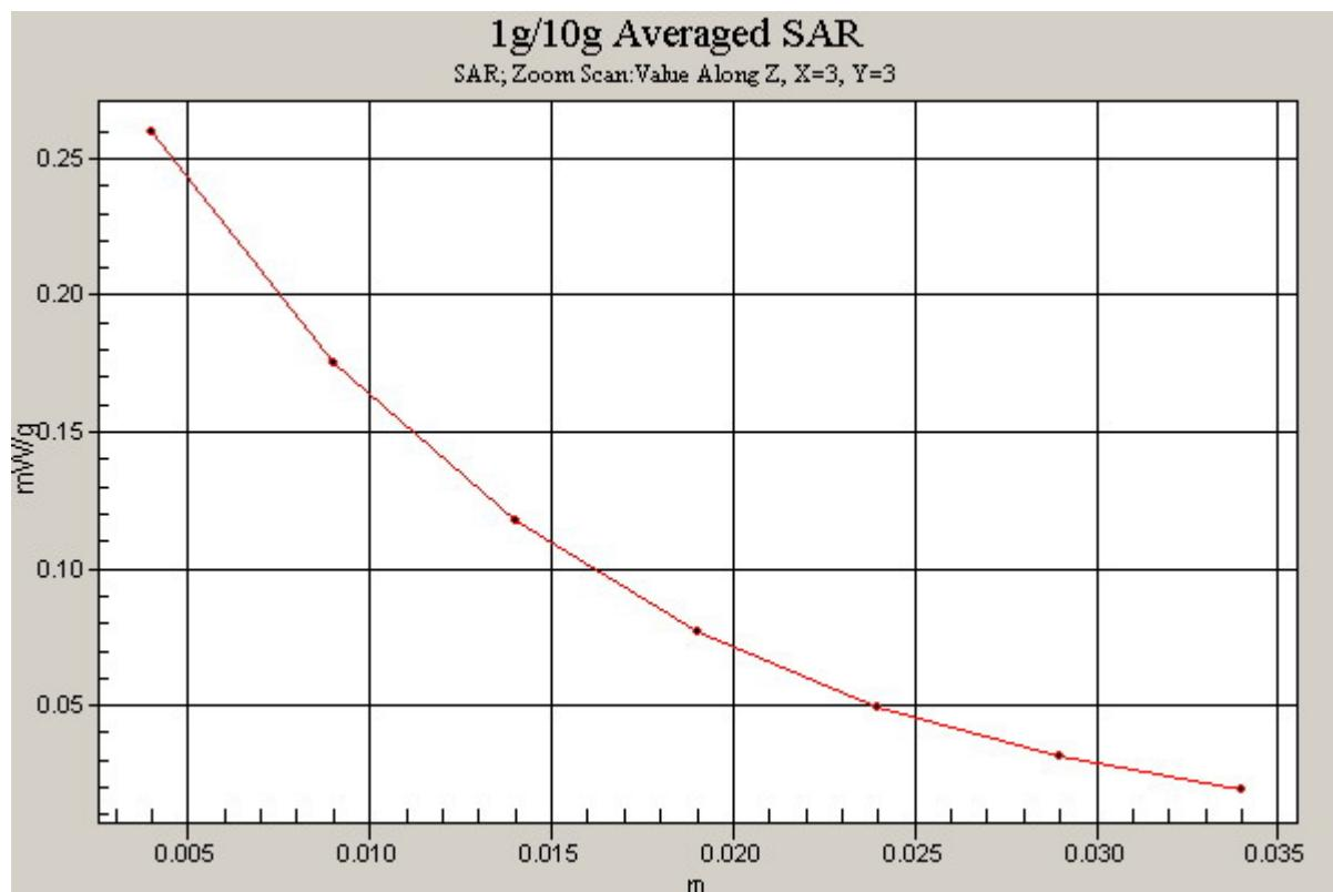
**Figure. 36 Z-Scan at power reference point (Body, Towards Phantom, CDMA PCS Channel 25)**
