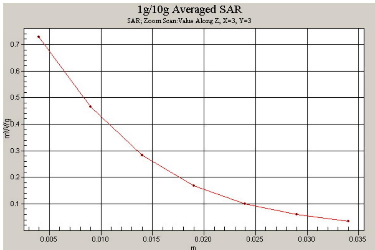
**Figure. 16 Z-Scan at power reference point (Left Hand Tilt 15° CDMA PCS Channel 600)**
