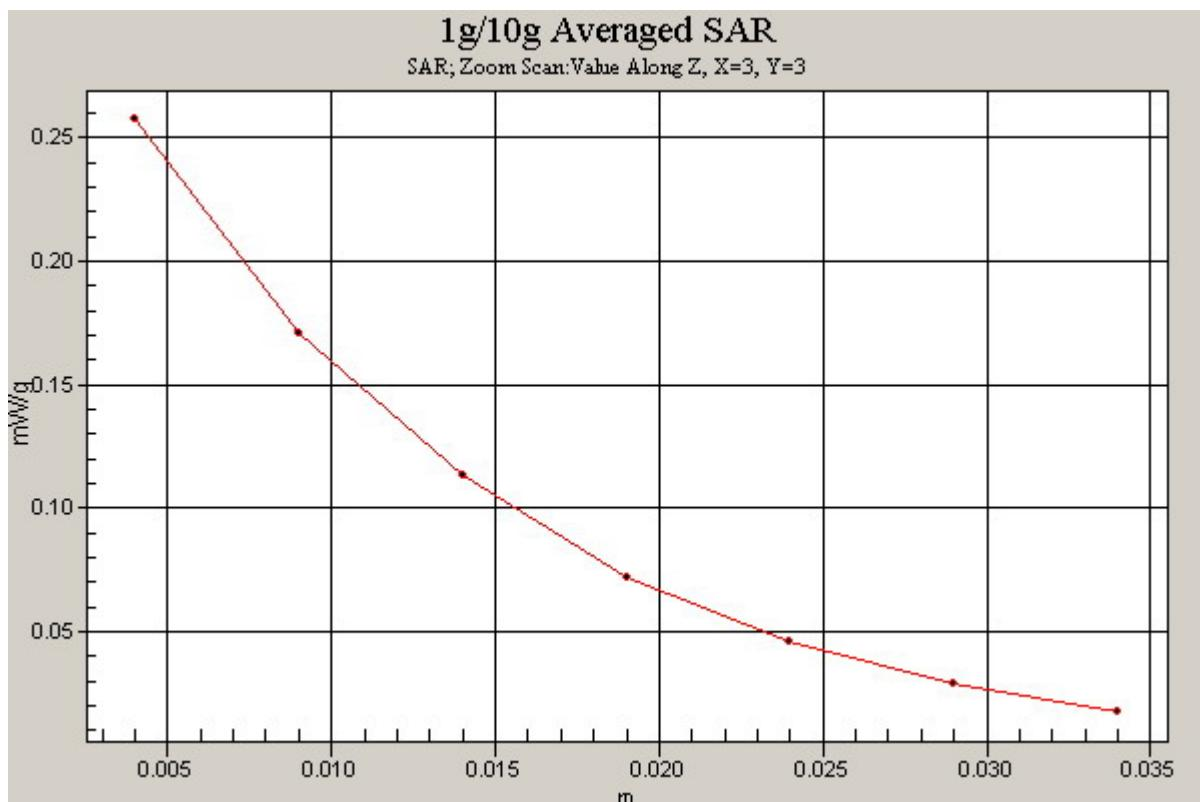
**Figure. 32 Z-Scan at power reference point (Body, Towards Phantom, CDMA PCS Channel 1175)**
