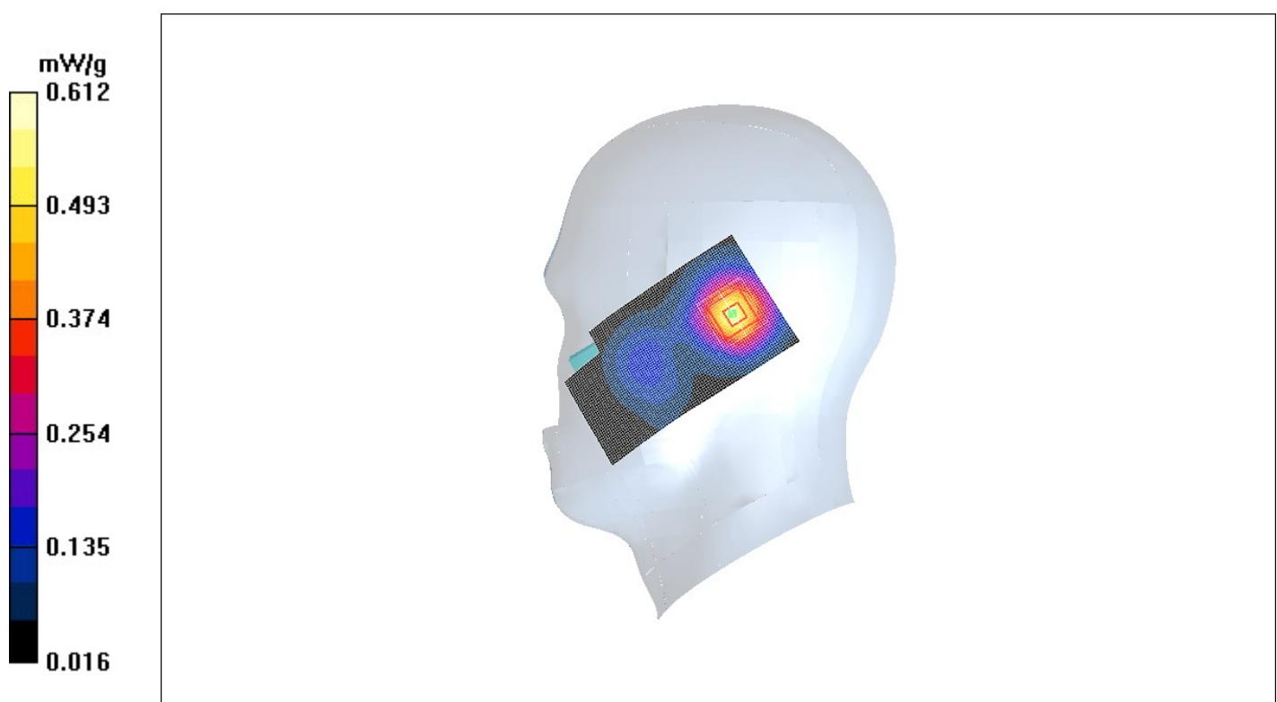
**Figure. 27 Right Hand Tilt 15° CDMA PCS Channel 600**
