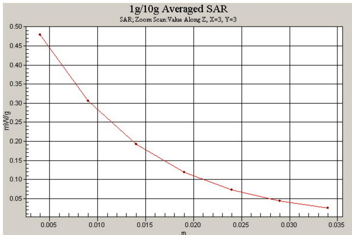
**Figure. 38 Z-Scan at power reference point (Body, Towards Ground, CDMA PCS Channel 1175)**
