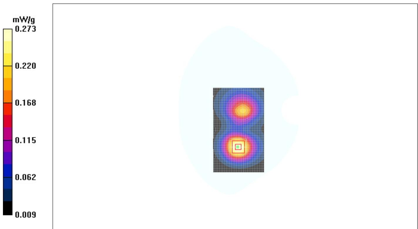
**Figure. 33 Body, Towards Phantom, CDMA PCS Channel 600**
