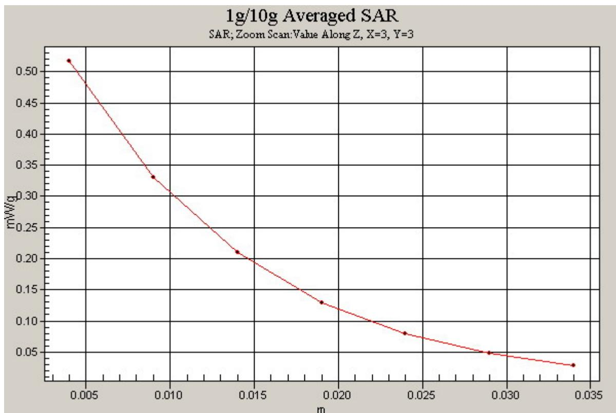
**Figure. 40 Z-Scan at power reference point (Body, Towards Ground, CDMA PCS Channel 600)**
