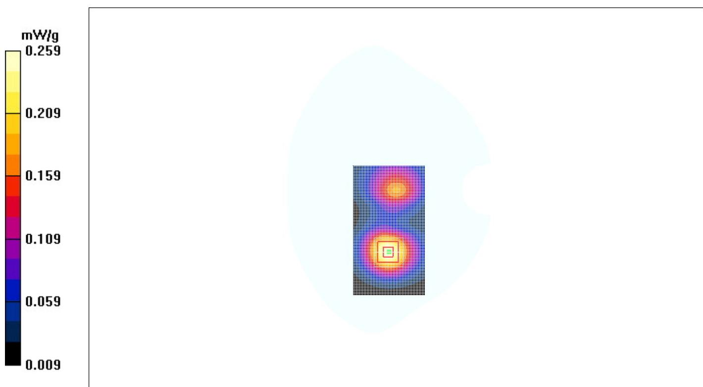
**Figure. 35 Body, Towards Phantom, CDMA PCS Channel 25**
