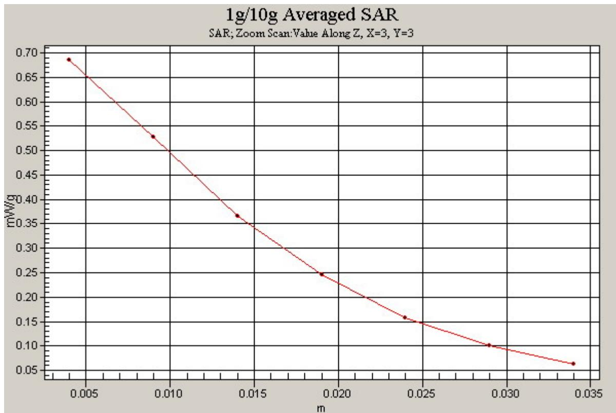
**Figure. 22 Z-Scan at power reference point (Right Hand Touch Cheek CDMA PCS Channel 600)**
