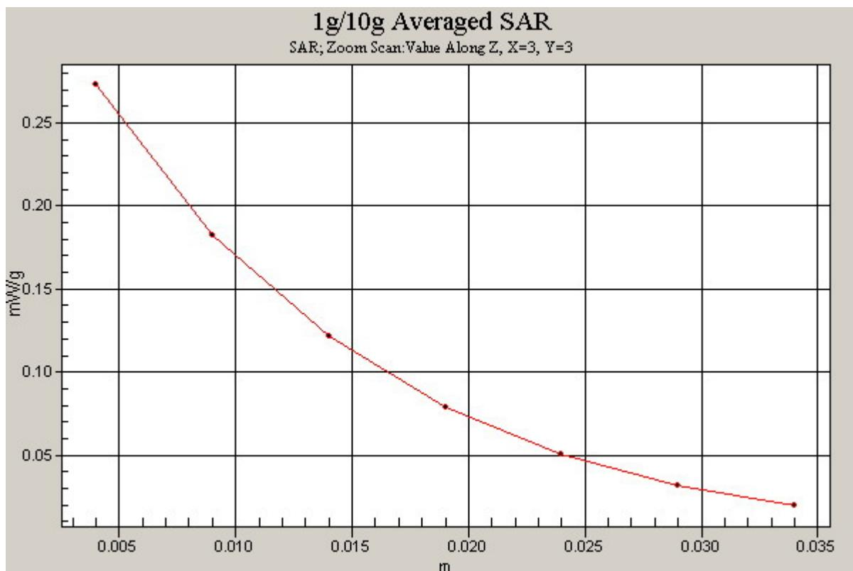
**Figure. 34 Z-Scan at power reference point (Body, Towards Phantom, CDMA PCS Channel 600)**
