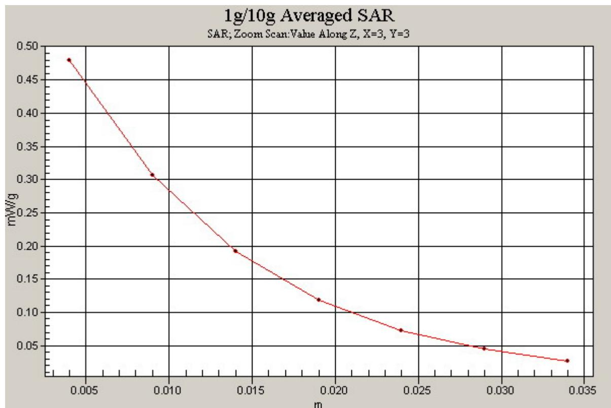
**Figure. 42 Z-Scan at power reference point (Body, Towards Ground, CDMA PCS Channel 25)**
