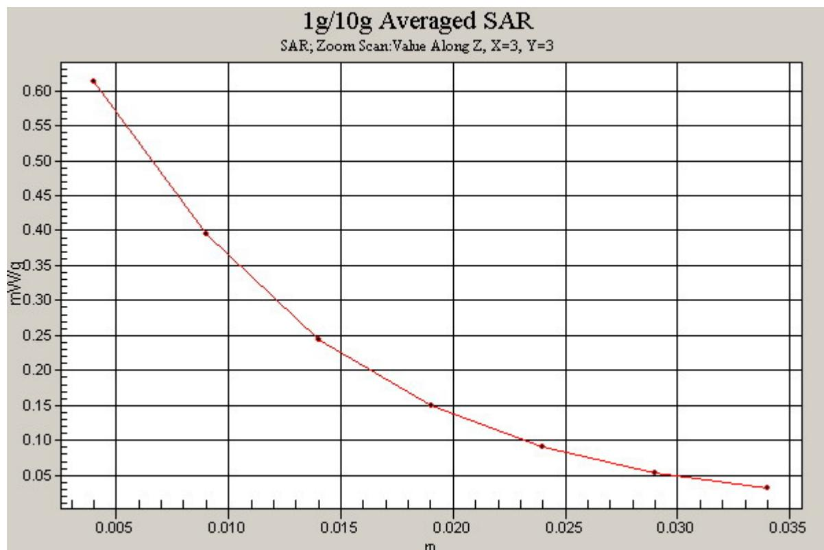
**Figure.28 Z-Scan at power reference point (Right Hand Tilt 15° CDMA PCS Channel 600)**
