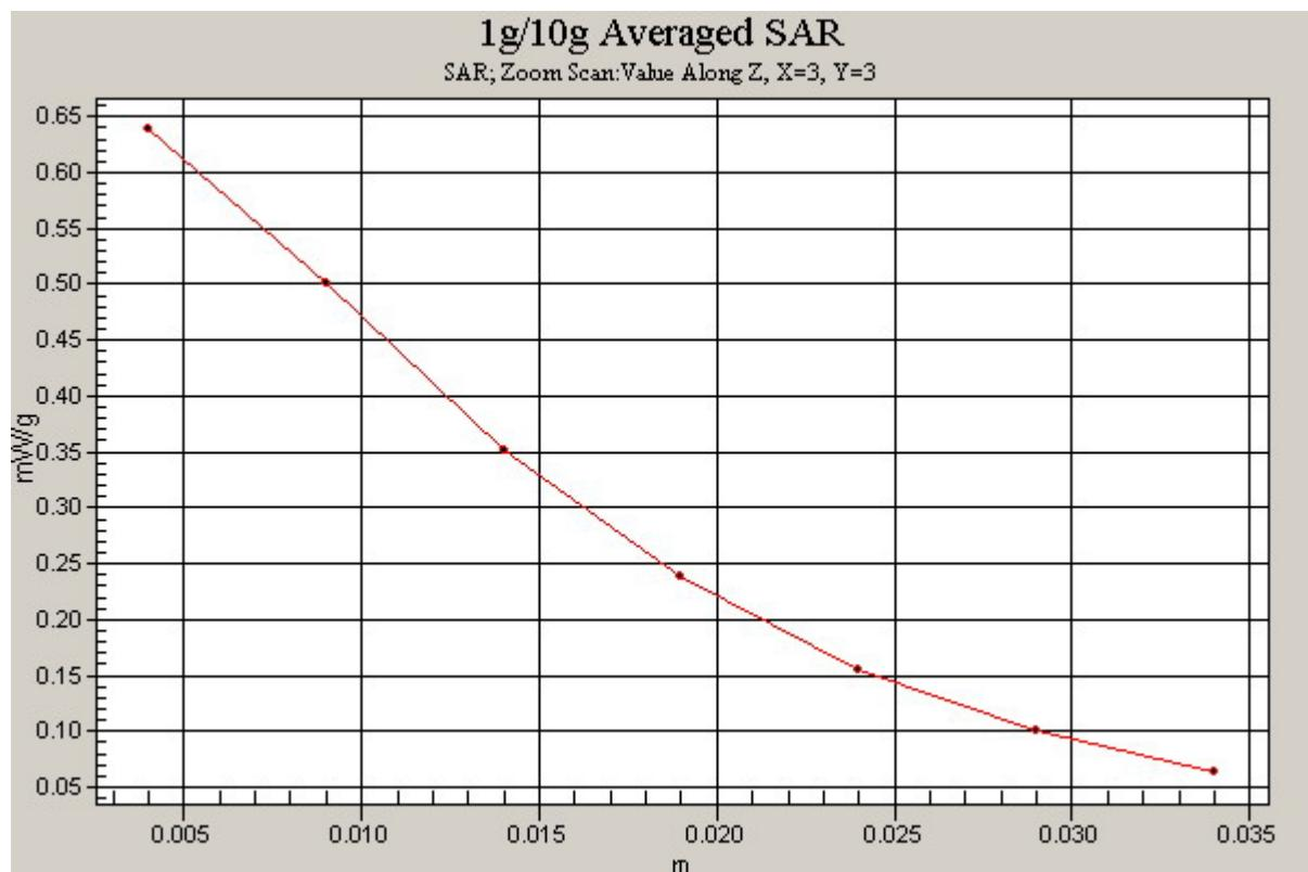
**Figure. 24 Z-Scan at power reference point (Right Hand Touch Cheek CDMA PCS Channel 25)**
