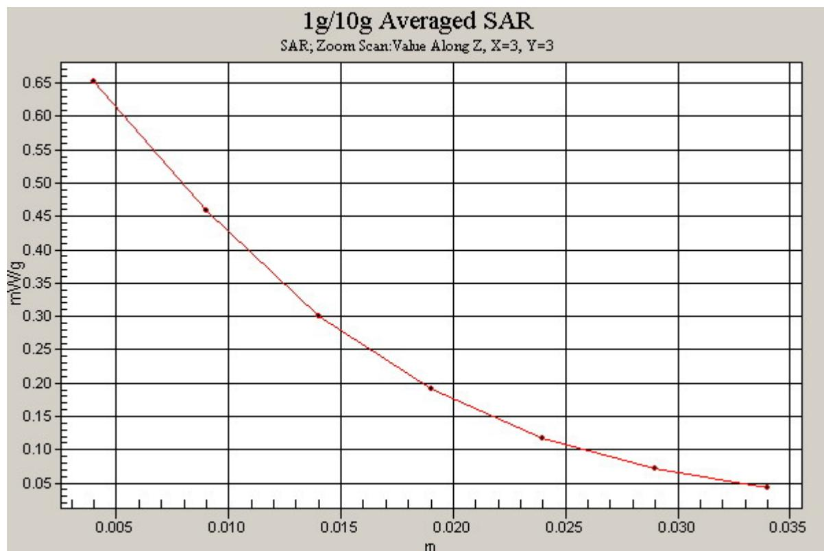
**Figure. 20 Z-Scan at power reference point (Right Hand Touch Cheek CDMA PCS Channel 1175)**
