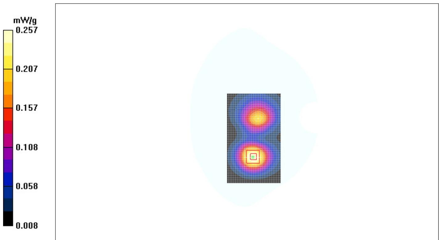
**Figure. 31 Body, Towards Phantom, CDMA PCS Channel 1175**
