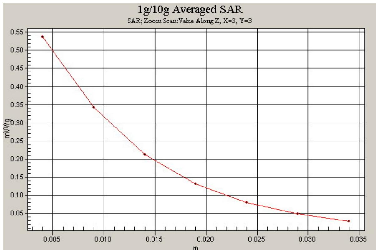
**Figure. 30 Z-Scan at power reference point (Right Hand Tilt 15° CDMA PCS Channel 25)**
