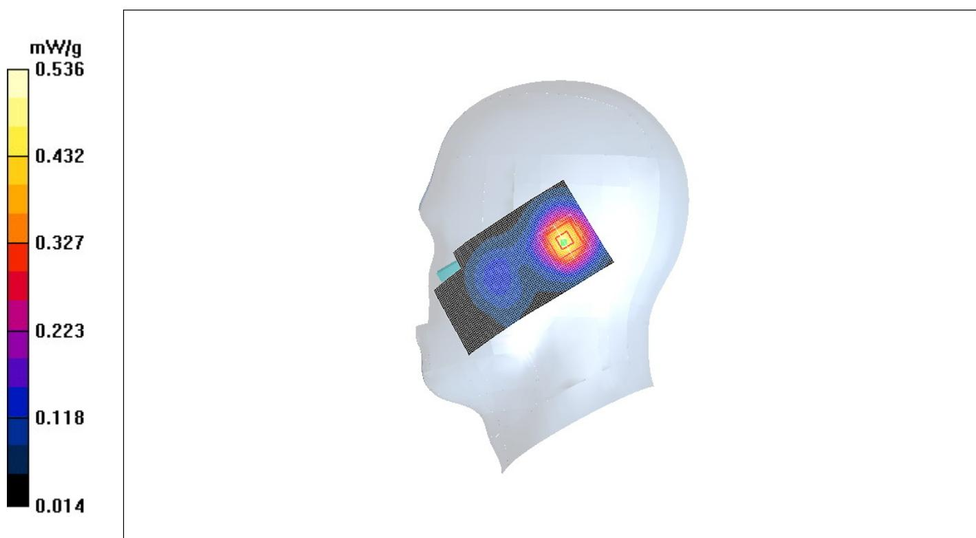
**Figure. 29 Right Hand Tilt 15° CDMA PCS Channel 25**
