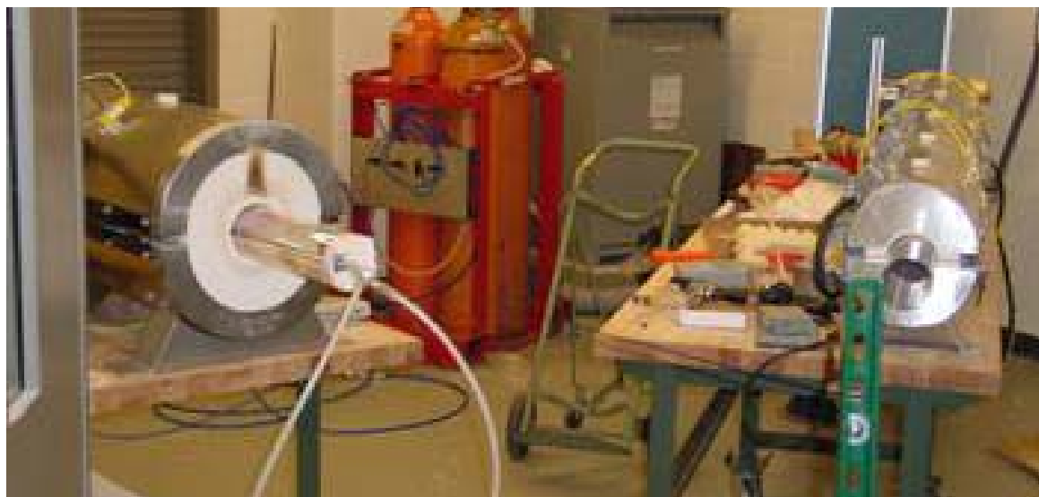
Figure 3. Continuous stabilization/oxidation (in furnace at right) and low-temperature carbonization (in furnace at left) of conventional 3k PAN precursor tow in precursor-evaluation system.
