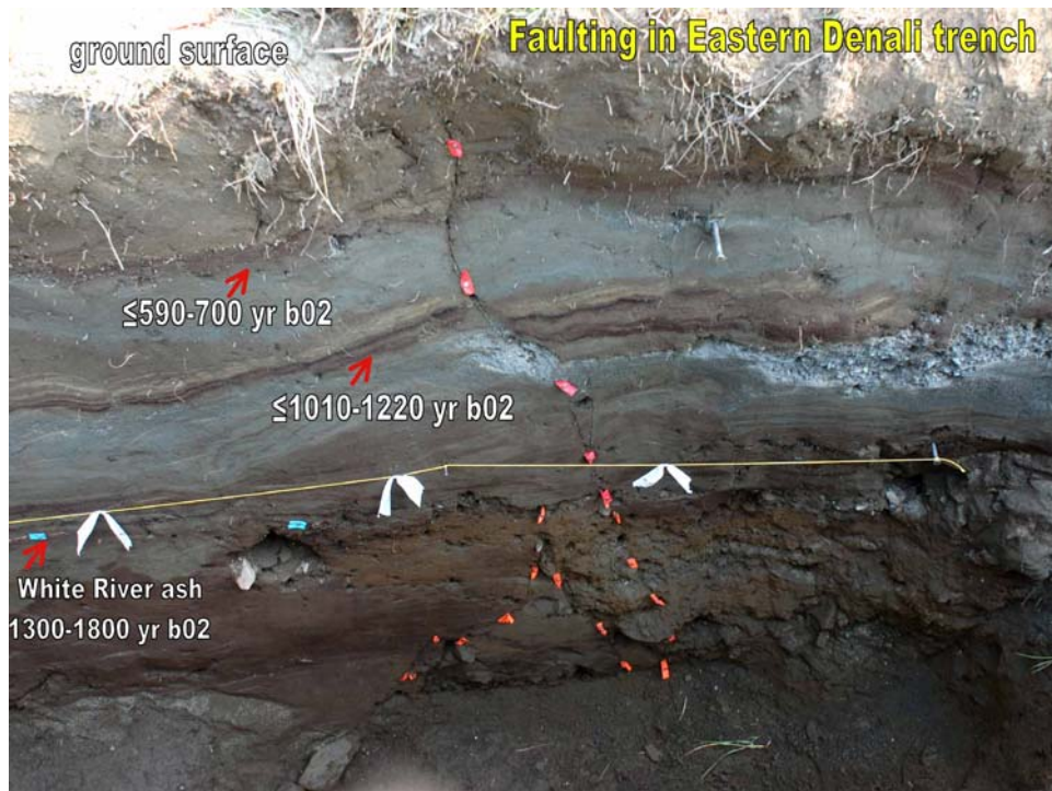
Figure 2. Photo of trench across the eastern unruptured Denali fault. The trench is 2m deep. Radiocarbon samples were collected during reconnaissance in July 2004 and dated prior to more extensive trenching in August 2004. Note broader zone of deformation at depth and rupture (orange flags) and the most recent event (red flags) extending to near the surface.
