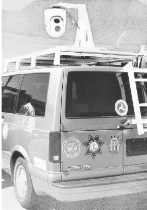
Figure A-1. The IRISystem, showing the housing minivan, and the camera mount on the roof (Photo courtesy of J. Bibb).
