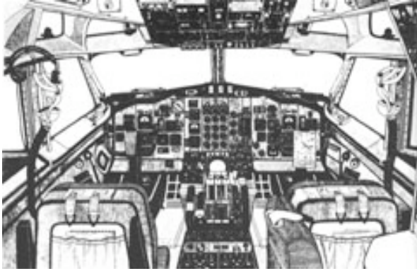
Figure 11. View of the forward panel of a 727 cockpit showing the artificial horizon on the attitude direction indicator. Two of these instrument may be seen directly in front of the control yokes. The lightly colored upper half disk on each shows the aircraft to be in level flight
