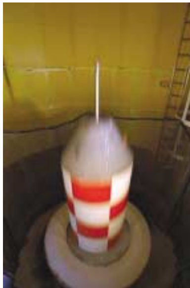
An experiment at the end of its fall inside the 5.2-second drop tower.
