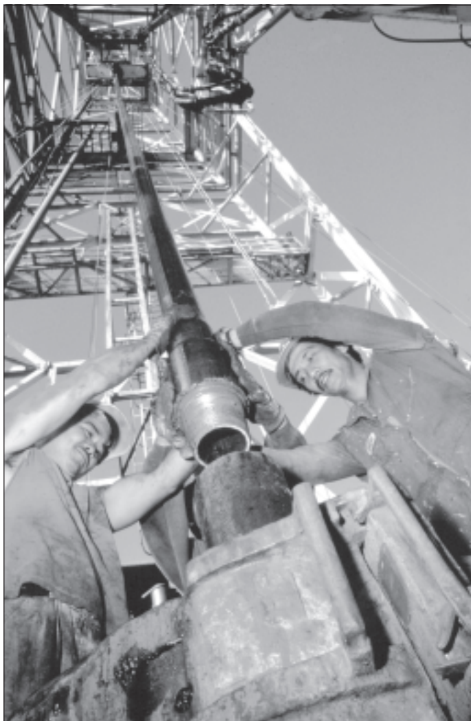
The ODP Rig Crew are connecting pipe.
