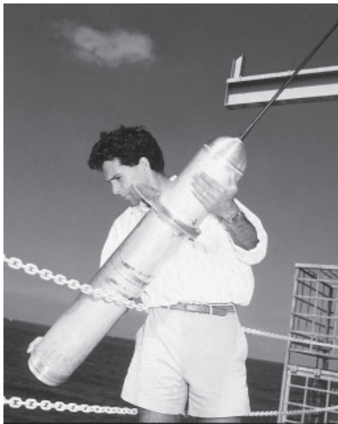
Profiling Autonomous Lagrangian Circulation Explorer (PALACE) float. Photo is courtesy of R. Davis, SIO.
