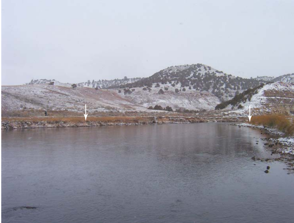
Figure B7. Tongue River at Tongue River Dam site from left bank looking upstream at cross section. Arrows indicate approximate bankfull elevation at cross section. Photograph taken October 23, 2002.
