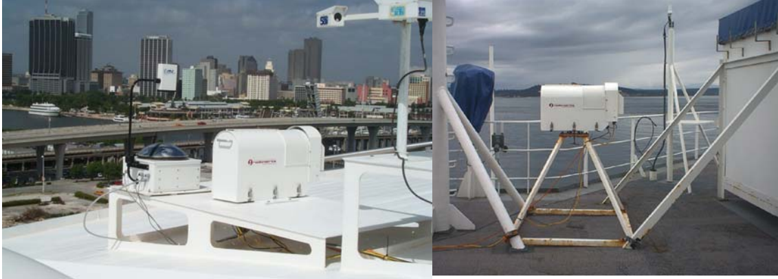
Figure 1. The Radiometrics MWR-100 microwave radiometer installed on the Explorer of the Seas (left) and on the USCGC Healy (right).
