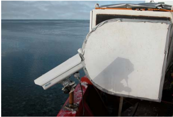
Figure 11. The M-AERI mounted on the NGCC Amundsen. The video camera housing forward of the M-AERI is used to record the conditions of the sea surface in the field of view, so that cases where ice is present, as is the case shown here, can be identified.
