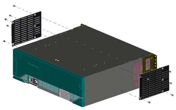
Figure 8 – 3845 – Opacity Shield Placement
