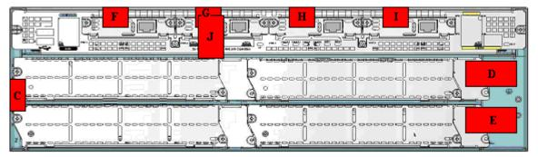
Figure 13 – Cisco 3845 Tamper Evident Label Placement (Back View)
