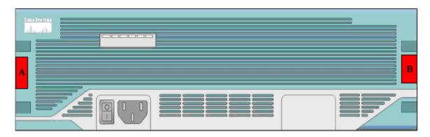
Figure 12 – Cisco 3845 Tamper Evident Label Placement (Front View)
