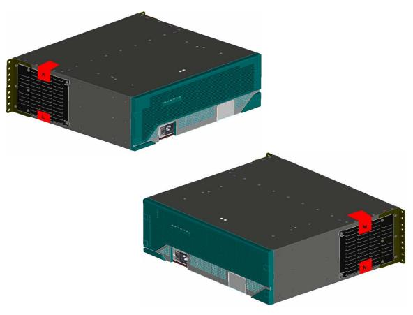
Figure 14 - Cisco 3845 Tamper Evident Label Placement (Side Views)
