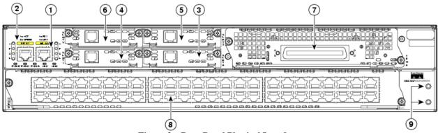
Figure 3 – Rear Panel Physical Interfaces
