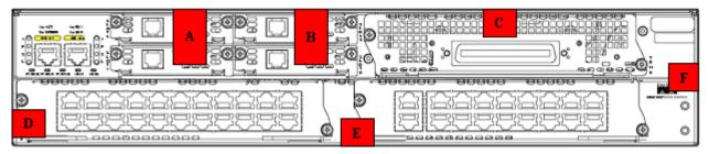
Figure 5 – 2851 Tamper Evident Label Placement (Back View)
