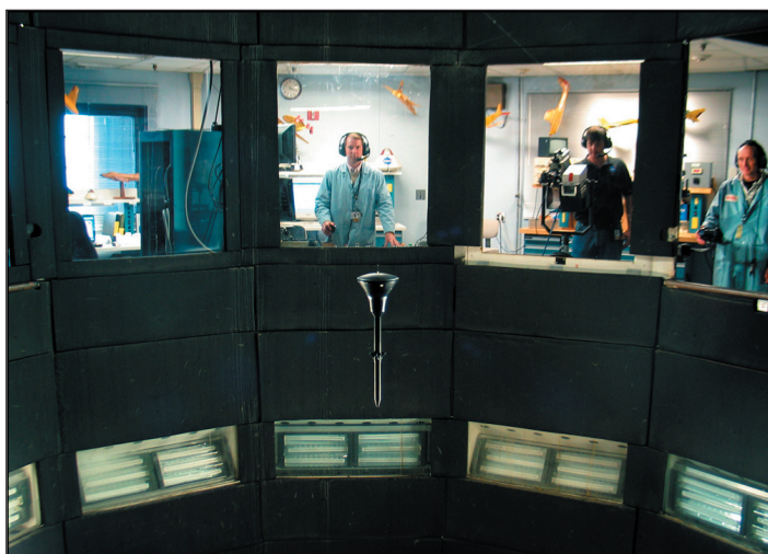
Researchers at NASA's Langley Research Center in Hampton, Va., conducted spin tunnel testing on a 1:29 scale model of the Launch Abort System in January.
