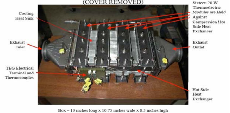
330 W THERMOELECTRIC GENERATOR FOR GM SIERRA 1999 TRUCK (COVER REMOVED)
