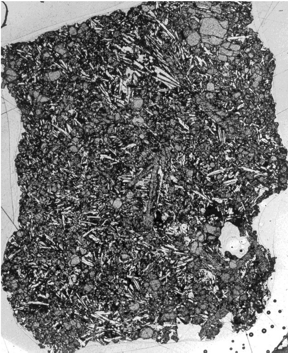
Figure 2: Photomicrograph of thin section 12020,13 illustrating round olivine and elongate pyroxene phenocrysts with variolitic intergrowths of plagioclase and pyroxene needles. NASA S70-30254. Field of view about 2 cm.
