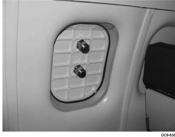
Figure 15. Dedicated Overboard Vent Ports
