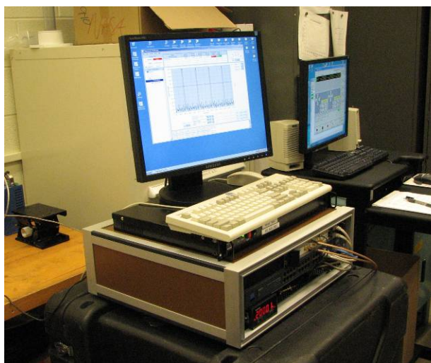
Figure 2. Microwave sensor electronics and data computer.
