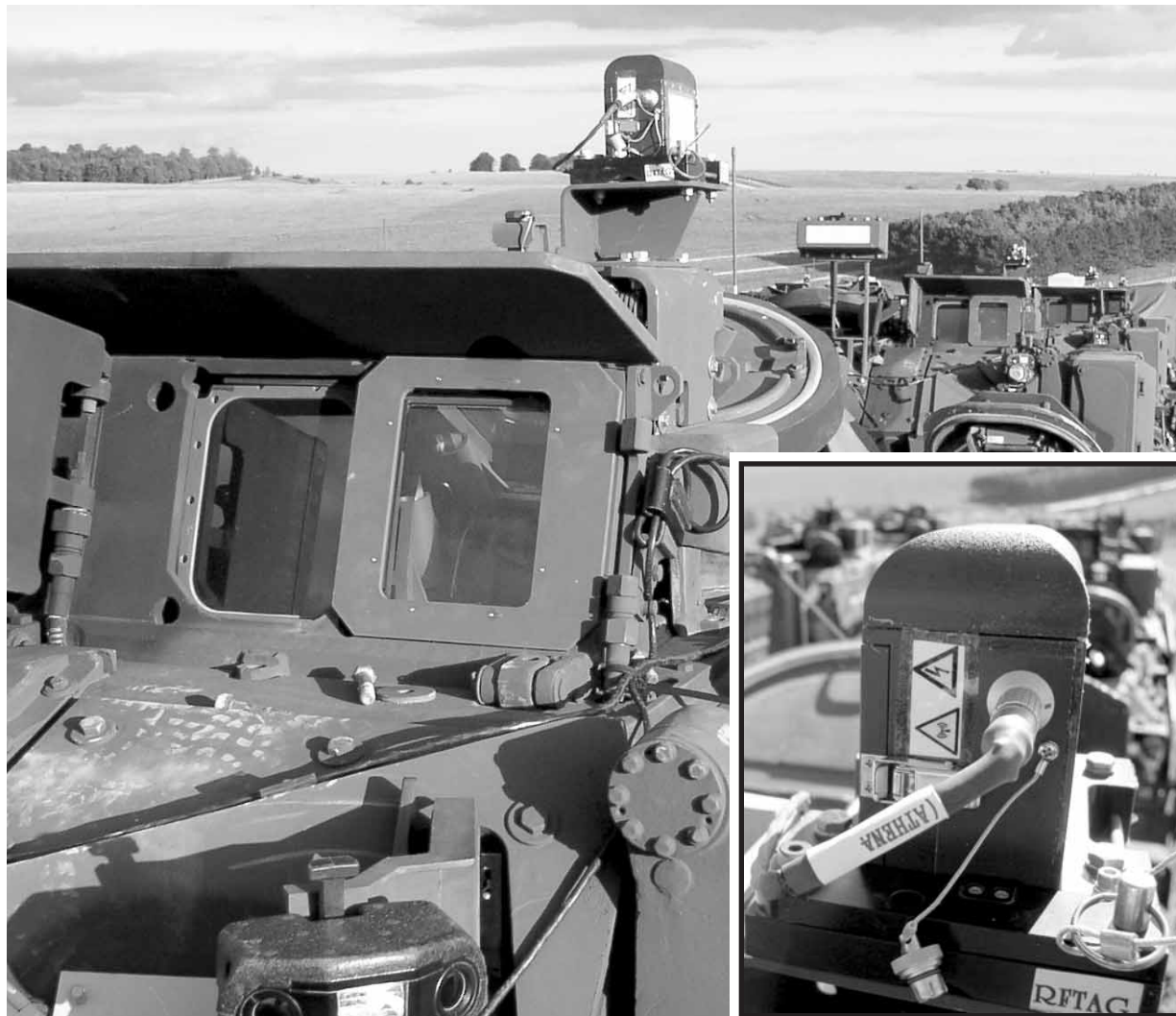
AN ARMORED VEHICLE deployed during Exercise Urgent Quest is seen here with the Athena tag mounted atop the roof, affording clear line of sight to friendly aircraft above. The Athena unit is shown in more detail in the inset photo.
