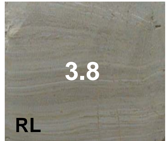
laminated silt loam
