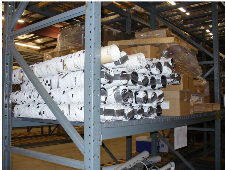
Figure 6.5. Photograph of preassembled thermistor bundles. Each bundle of 24 thermistors is spooled on a PVC spindle for minimize tangling and simplify installation
