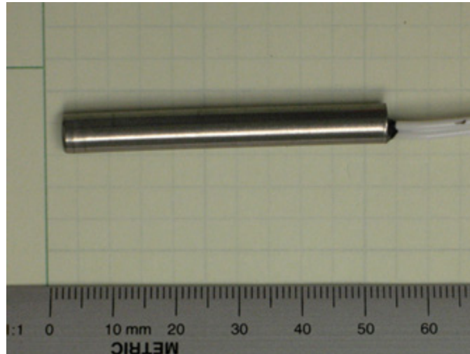
Figure 6.4. Photograph of potted thermistor that will be used for in situ temperature measurements
