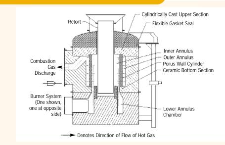
The new PWRB heating mantle offers increased heat-transfer rates, increased energy savings, and a significant reduction in emissions.
