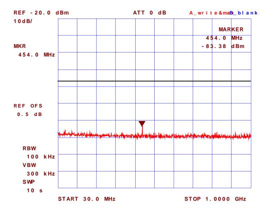
Plot #4: Receiver Antenna Power Conducted Emissions Receive Frequency: 30 MHz
