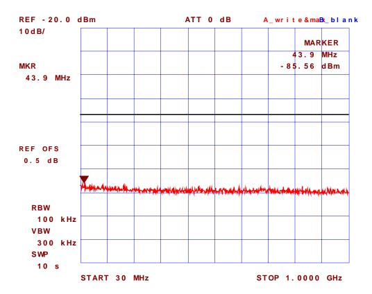
Plot #8: Receiver Antenna Power Conducted Emissions Receive Frequency: 960 MHz
