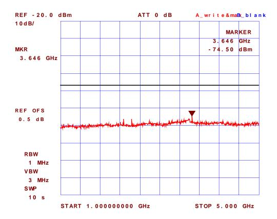
Plot #5: Receiver Antenna Power Conducted Emissions Receive Frequency: 495 MHz
