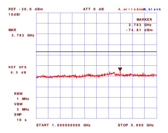
Plot #7: Receiver Antenna Power Conducted Emissions Receive Frequency: 960 MHz
