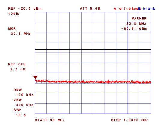
Plot #6: Receiver Antenna Power Conducted Emissions Receive Frequency: 495 MHz
