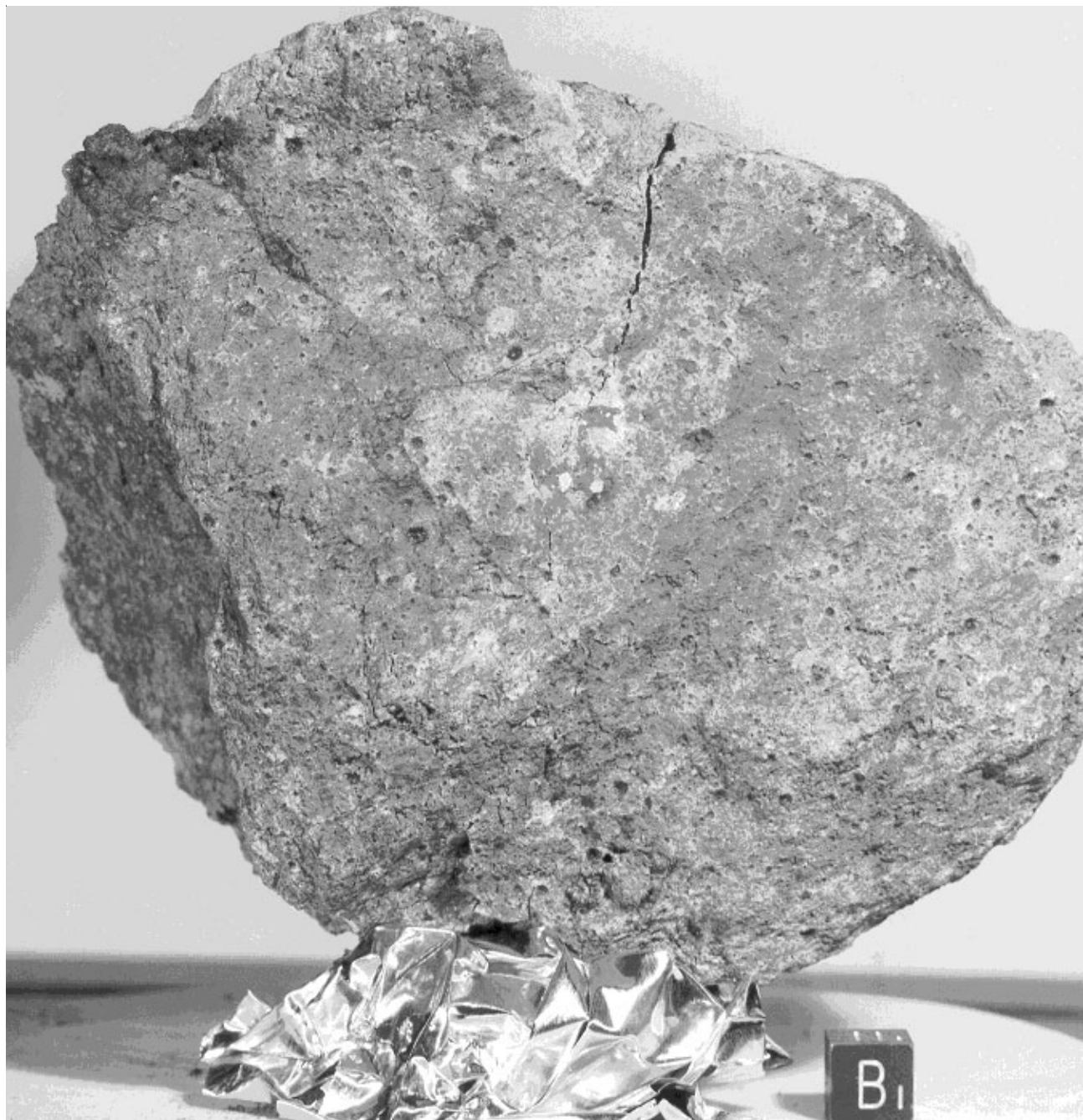
Figure 1: Photo of top surface of 66095 (note the zap pits and penetrating fracture). Cube is 1 cm. NASA S72-41445.
