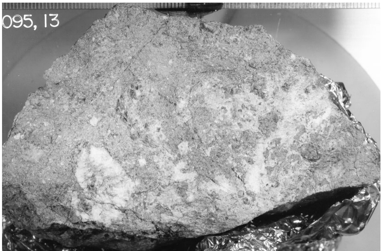
Figure 6: Photo of freshly broken surface of 66095,13, showing anorthosite clast and region of mixed anorthosite and melt rock material. Sample is 11 cm across. NASA S79-34547.
