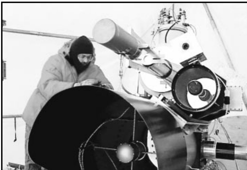
Fred Mrozek makes adjustments to the Spirex infrared telescope, which he built by hand. SPIREX is one of three telescopes at the South Pole, a location some Astronomers are calling the next place where astrophysics will take-off.
