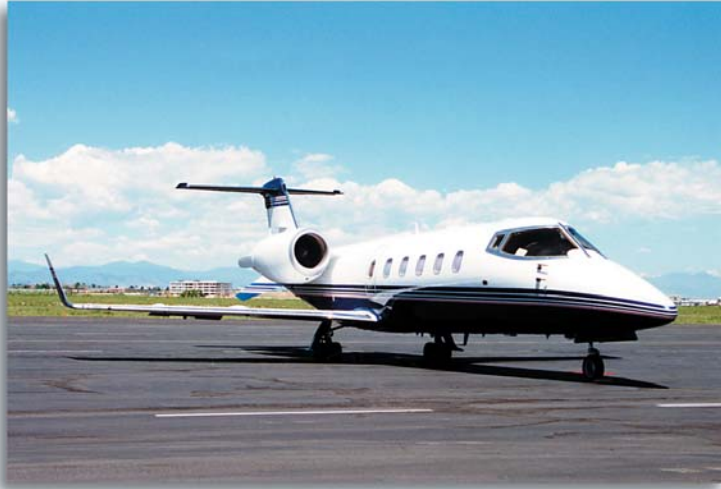
The winglets on this Learjet help reduce induced drag.
