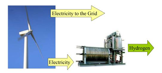
Figure 3: Grid Connected Wind/Hydrogen Plant
