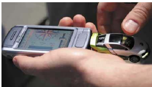
Computer Science students at Armstrong Atlantic used J2ME to wirelessly control a Bluetooth equipped racecar from a cell phone. The project combined cutting edge Bluetooth wireless technology to control the miniature racecar with cell phone programming to create the control application.
