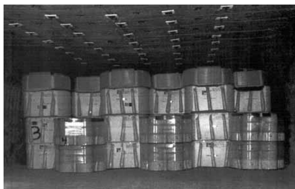
TRANSURANIC WASTE in seven packs and standard waste boxes are stacked three high and topped with a super sack of magnesium oxide.
