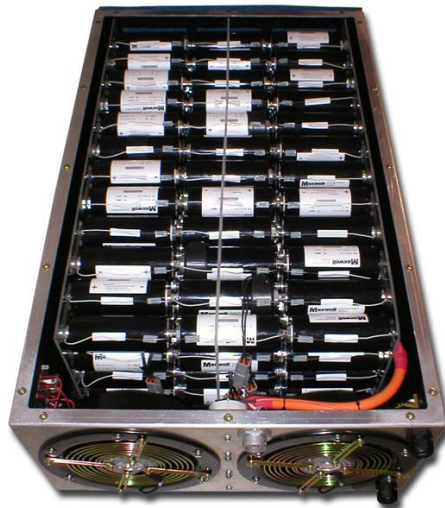
Figure 9. An Open ultra-capacitor pack.
