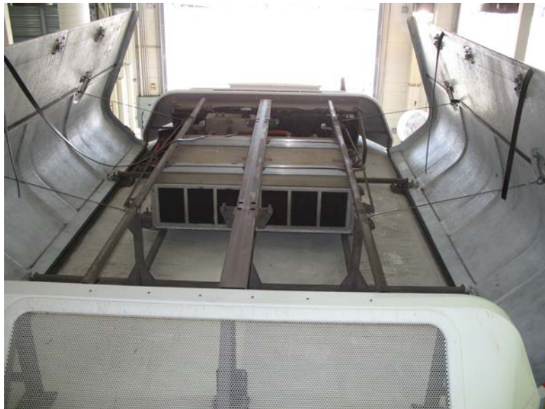
Figure 9. An Open ultra-capacitor pack.
