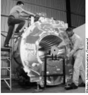
A large-bore superconducting magnet, built by Intermagnetics General Corporation, destined for a magnetic resonance imaging system.
