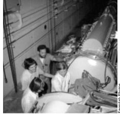
Scientists had to install a magnet in the beamline of the already existing linear accelerator to extract proton beams and direct them to the neutron production target.
