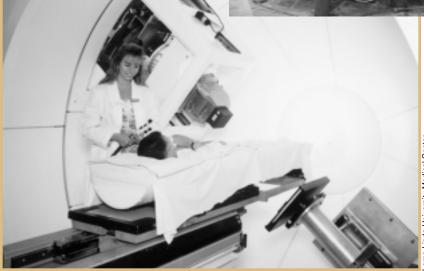
Loma Linda University Medical Center uses the world's first proton accelerator built specifically to administer proton therapy in a medical environment. The synchrotron accelerator was built at Fermilab and shipped to Loma Linda, where the first patients were treated in 1990. Since then, more than 6,000 patients have been treated. Loma Linda researchers are now intensifying their efforts to apply proton therapy to breast cancer.
