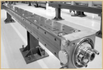
Fermilab's Tevatron accelerator is a four-mile circle of 1,020 superconducting magnets, 224 quadrupoles, like this one, and 796 dipoles. Building the Tevatron took enough superconducting wire to circle the earth 2.3 times-and created a new industry, ready to supply superconducting wire and cable for the emerging medical technology called magnetic resonance imaging.
