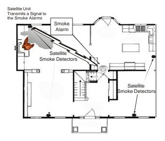
Figure 8. Satellite Smoke Detector Units
