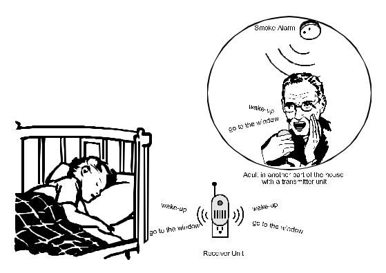
Figure 10. Remote Alerting System
