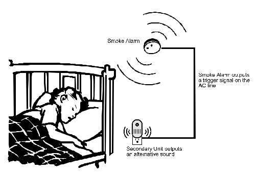
Figure 7b. Secondary Unit Triggered by Signal on the AC Line
