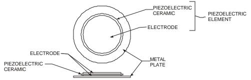
Figure 1. Piezoelectric Diaphragm
