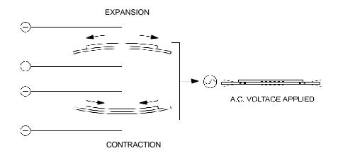
Figure 2. AC Voltage Applied to the Piezoelectric Element
