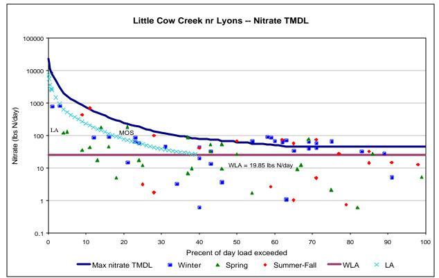
allocation calculations are strictly based on the design flow (0.85 cfs) of the Lyons wastewater treatment plant.
