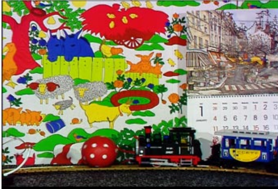
Figure 1: Mobile and Calendar is challenging to MPEG compression. Mosquito noise is produced in image regions with sharp edges, such as in the lettering.
