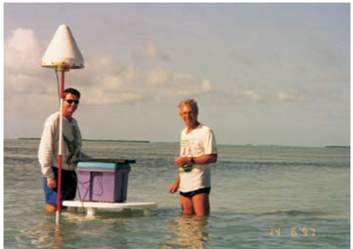
USGS St. Petersburg scientists setting up a Real-Time Kinematic (RTK) Global Positioning System (GPS) receiver.
