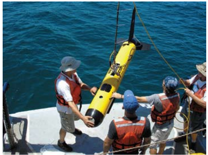
USGS and University of South Florida (USF) researchers deploy C3D sidescan system to map water depth and bottom characteristics in the Gulf of Mexico.
