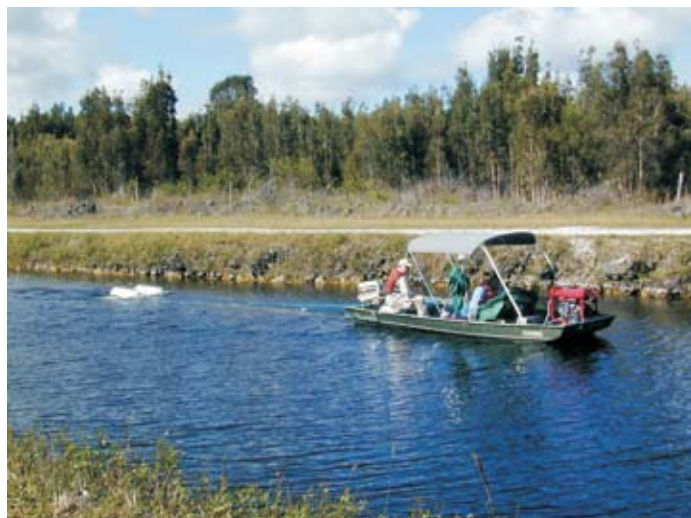
Jon boat towing seismic "boomer" equipment to map bathymetry of an inland canal in Florida.
