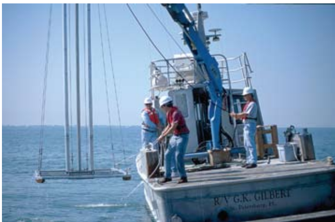
Vibracore system being lowered from the R/V Gilbert. The sediment core is used to ground-truth seismic data.
