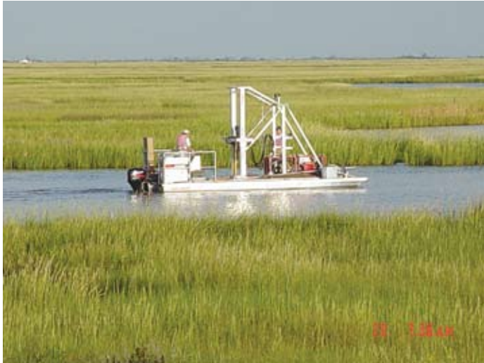
Pontoon barge carrying the Portable Auger Drilling System (PADS).
