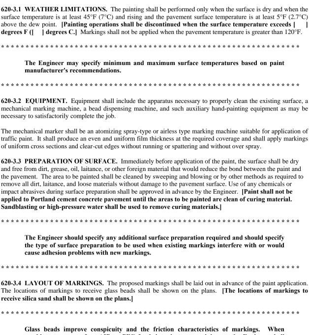
Glass beads improve conspicuity and the friction characteristics of markings. When markings are part of an AIP or PFC funded project, at a minimum, the Engineer shall indicate the following locations to receive glass beads:
