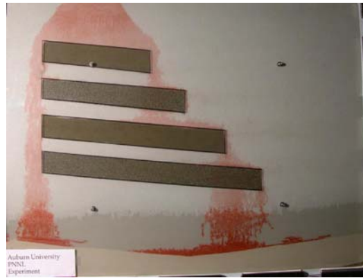
Figure 4. Near the final DNAPL distribution, full collapse of the capillary fringe was observed. This collapse was attributed to a reduction of the surface tension of water caused by DNAPL diffusion in the liquid phase.
