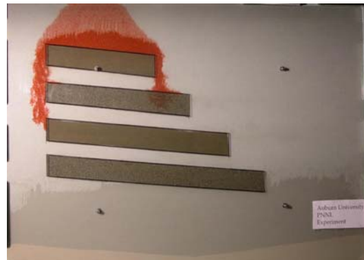
Figure 2. When the DNAPL reached the first layer (fine material), it spread to the left and right and then edged over both ends. When it reached the second layer (course material) on the right, the DNAPL moved through the layer.
