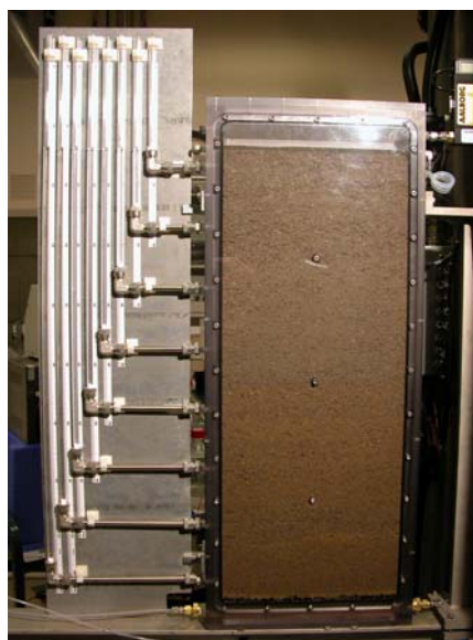
Figure 2. The pressure monitoring flow cell has several monometer ports to measure the build-up of gas pressures.
