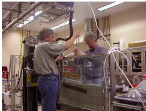
Figure 1. The Subsurface Flow and Transport Experimental Laboratory enables novel flow and transport studies. Here, scientific consultant Mark Oostrum, PNNL, and user Jacob Dane, Auburn University, Auburn, Alabama, prepare an experiment to investigate a complex dense nonaqueous phase liquid (DNAPL) – a composition similar to the mixture disposed of at the Hanford site in the 1950s and 1960s and now present in Hanford subsurface heterogeneous materials.
