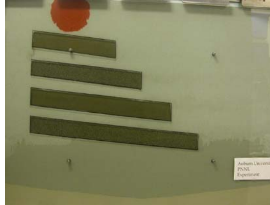
Figure 1. The four sloping layers, from top to bottom, consisted of fine, coarse, fine, and coarse material. The red sphere is the initial simulated DNAPL spill.
