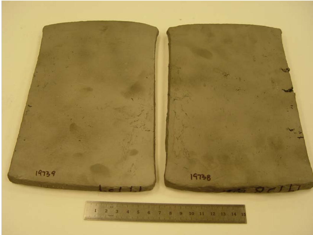
Figure 2. Hot rolled experimental heats of CMS alloy 617 (GenIV-7 heat is on the left and GenIV-6 is on the right)
