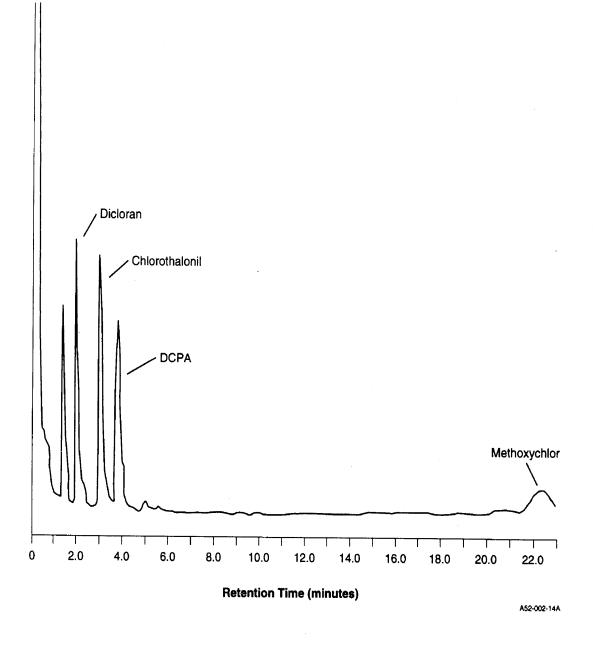
Figure 1. Gas Chromatogram of Chlorothalonil, DCPA, Dicloran, and Methoxychlor in a Wastewater Extract (Column 1)
