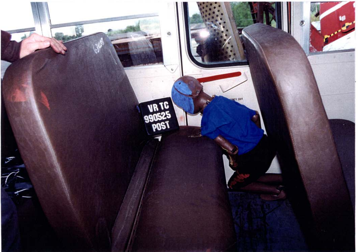
Figure A-38 Post-Test Left Side Seat 9 Ballast 6 Year Old - View 2
