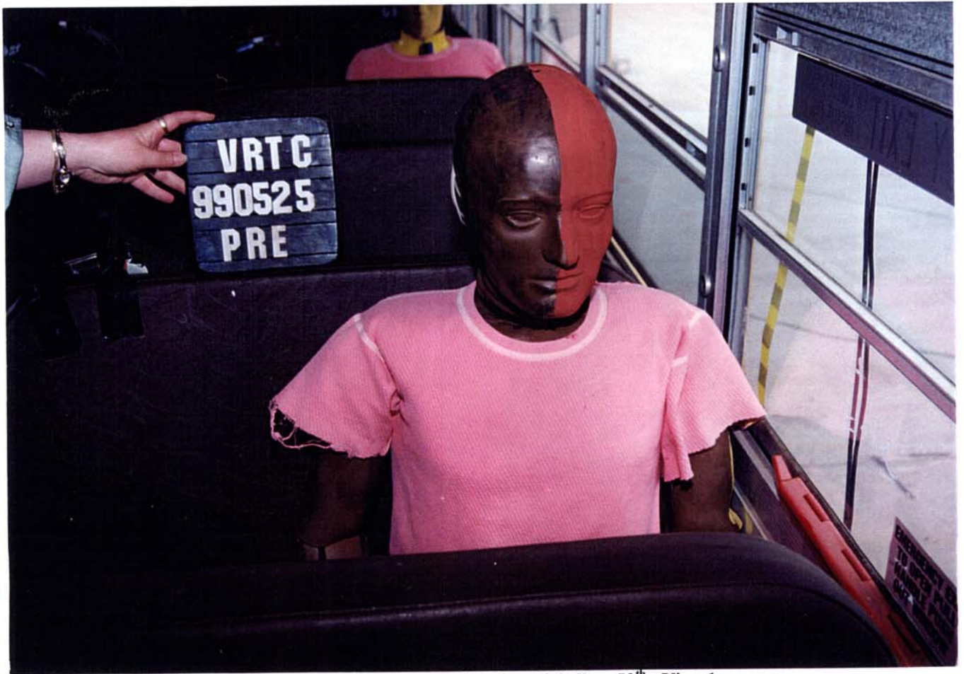
Figure A-12 Pre-Test Left Side Seat 4 Ballast 50 th - View 1
