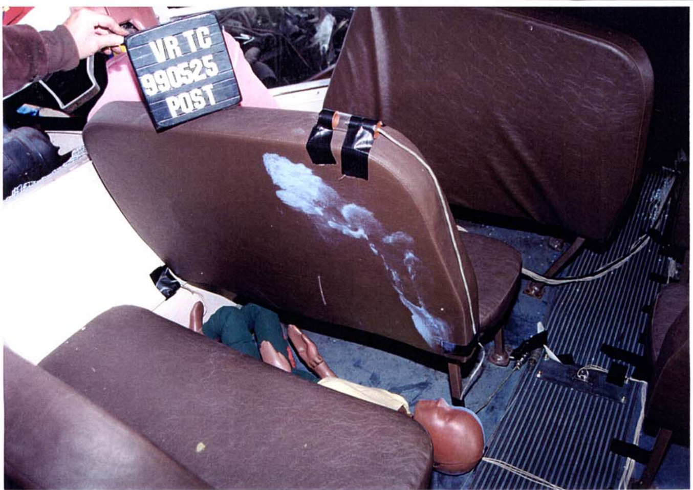
Figure A-43 Post-Test Right Side Seat 8 Ballast 6-year-old - View 1
