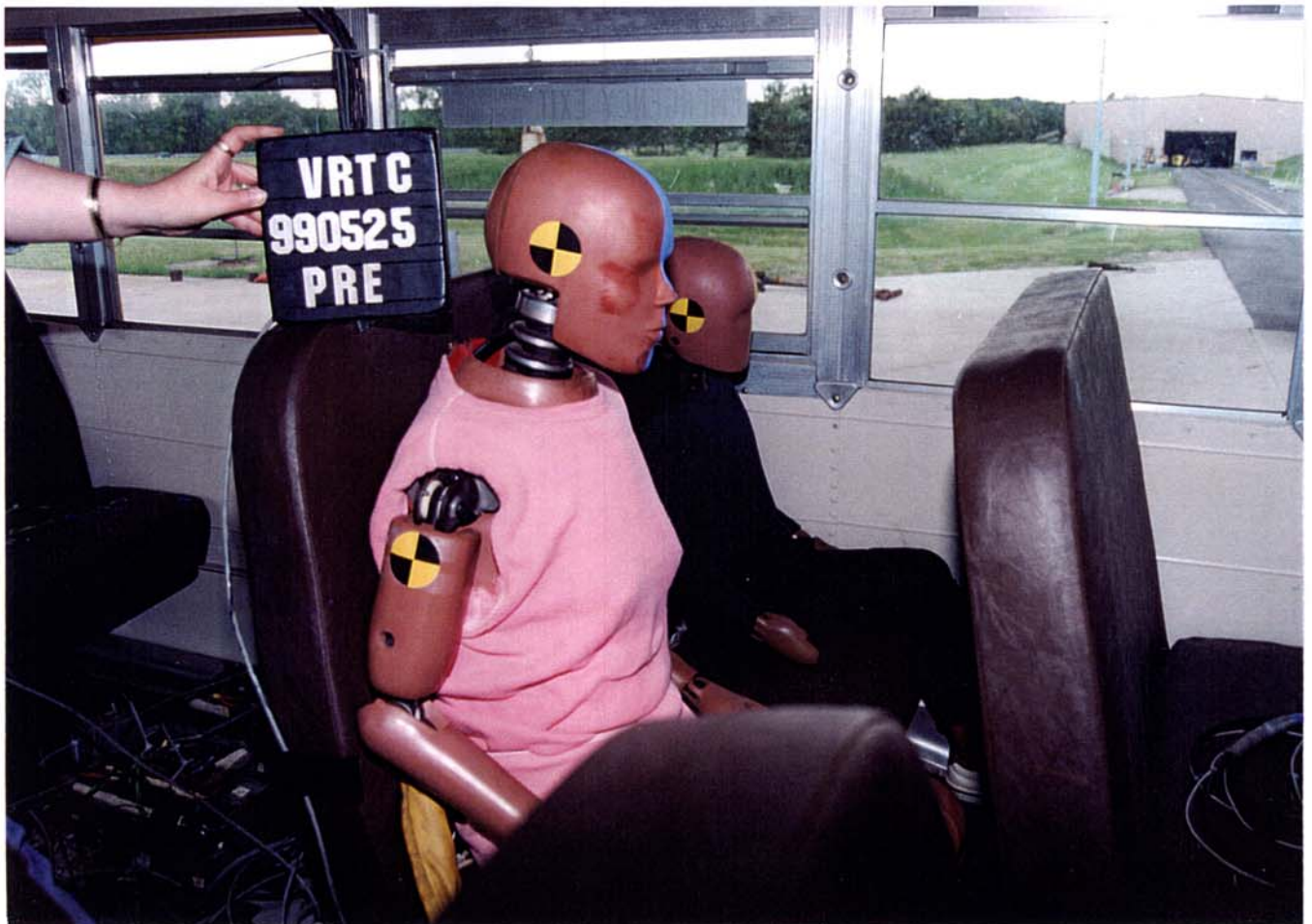
Figure A-19 Pre-Test Left Side Seat 11 Instrumented 5 th and 6 Year Old - View 2
