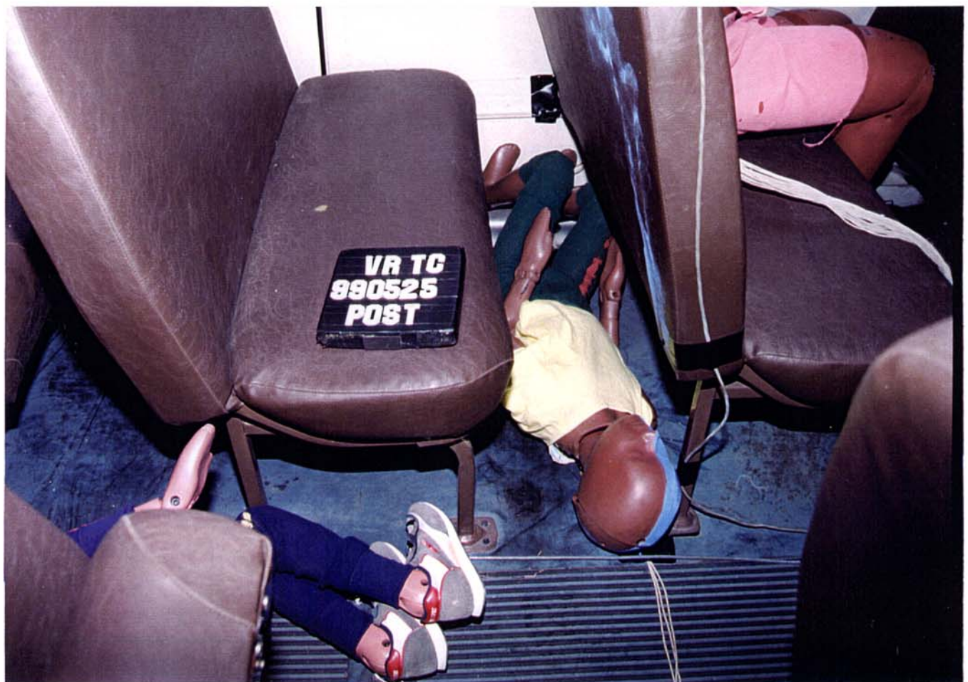
Figure A-44 Post-Test Right Side Seat 8 Ballast 6-year-old - View 2
