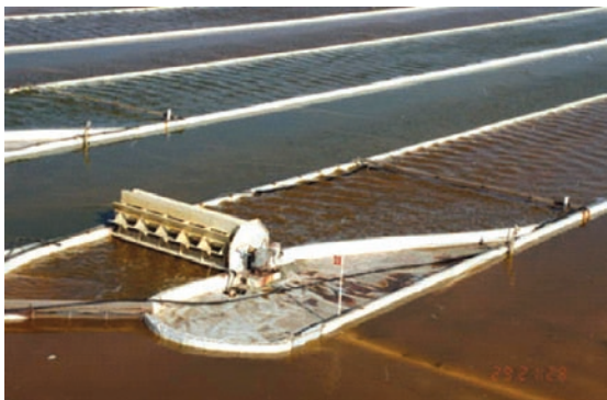
A raceway pond system in Israel growing microalgae for nutraceutical production. PIX 08332
