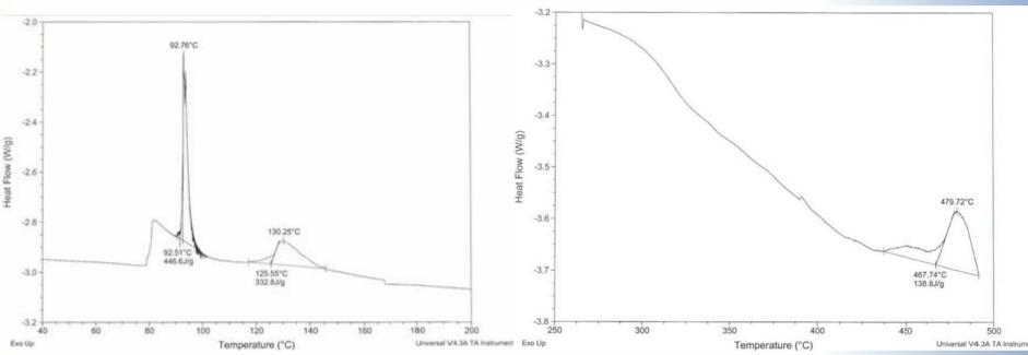
Release of heat during first stage, close to AB m.p., causes foaming and expansion of solid mass
