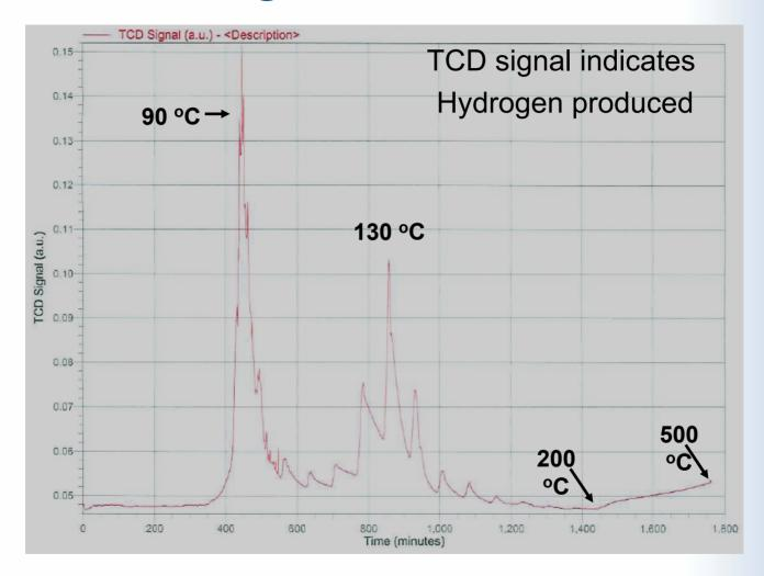
hydrogen released in slow heating ~ 67% in first two stages, ~ 1% in the third stage
