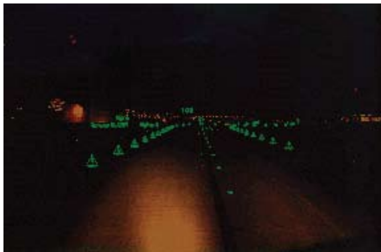
Figure 1: Head-up display depicted roll-out, turn-off, and taxi guidance
