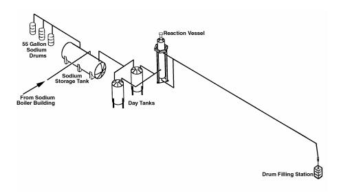
Fig. 3. Sodium Process Facility Flow Diagram
