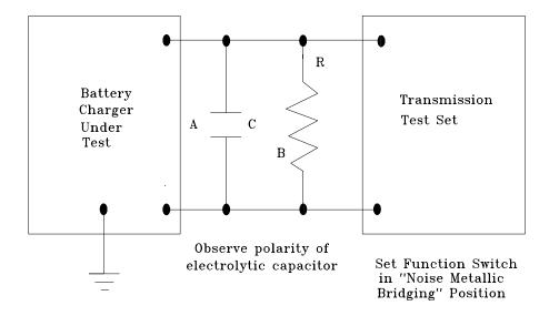
The manufacturer may elect to eliminate the capacitor C from the measurement.
