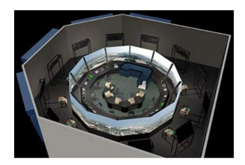
The 3D model was based on computer aided design (CAD) data provided by the airport engineering department. It was overlaid with realistic details of the terminal area, landscape, and distant cityscape using high-resolution photo textures. (Figure 2).
